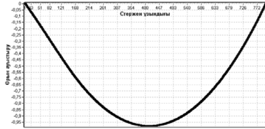
Figure-3 - The law of distribution of displacements of nodal points along the length of the rod with q = -70(W/cm^2)
